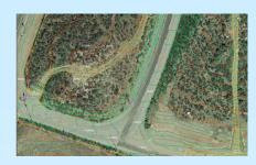
The purpose of a TOPOGRAPHIC SURVEY is to gather survey data about the natural and man-made features of the land, as well as its elevations. From this information a three-dimensional map may be prepared. You may prepare the topographic map in the office after collecting the field data by GPS or Total Station.
